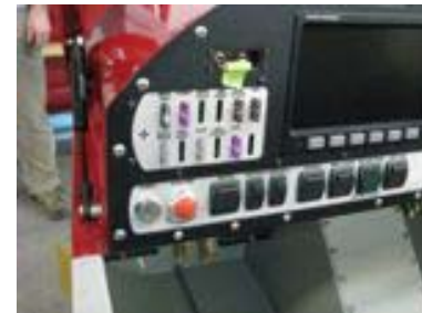
Switch and Fuse detail
